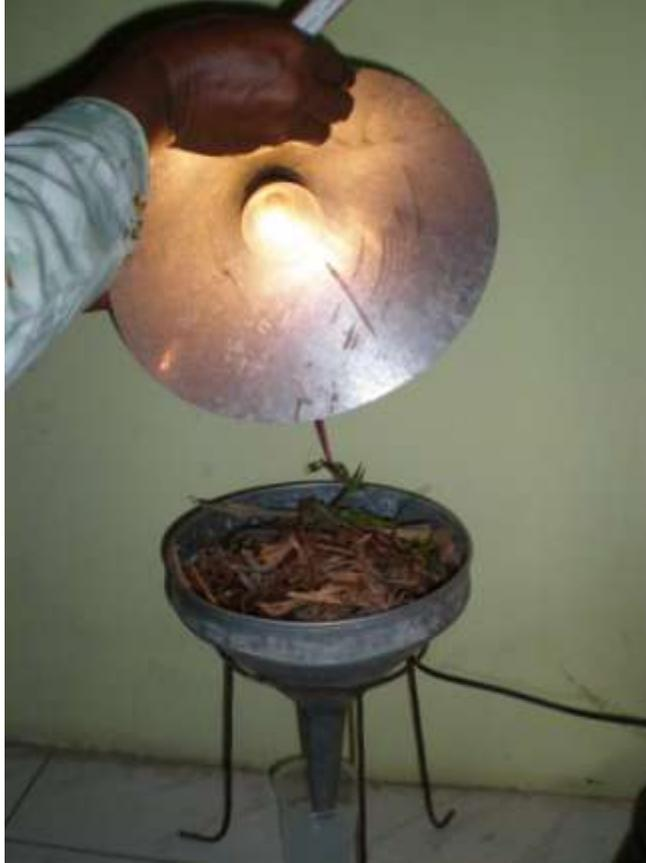
Picture: Funnel cup with humus inside and electric lamp of 25 watts
