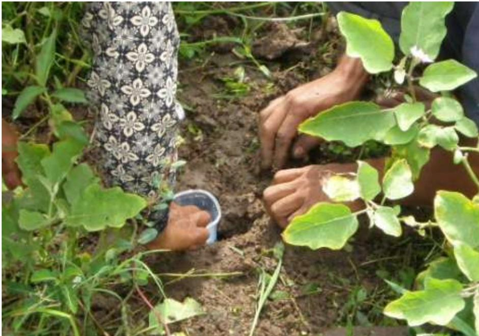
Picture: Pitfall cup installation
